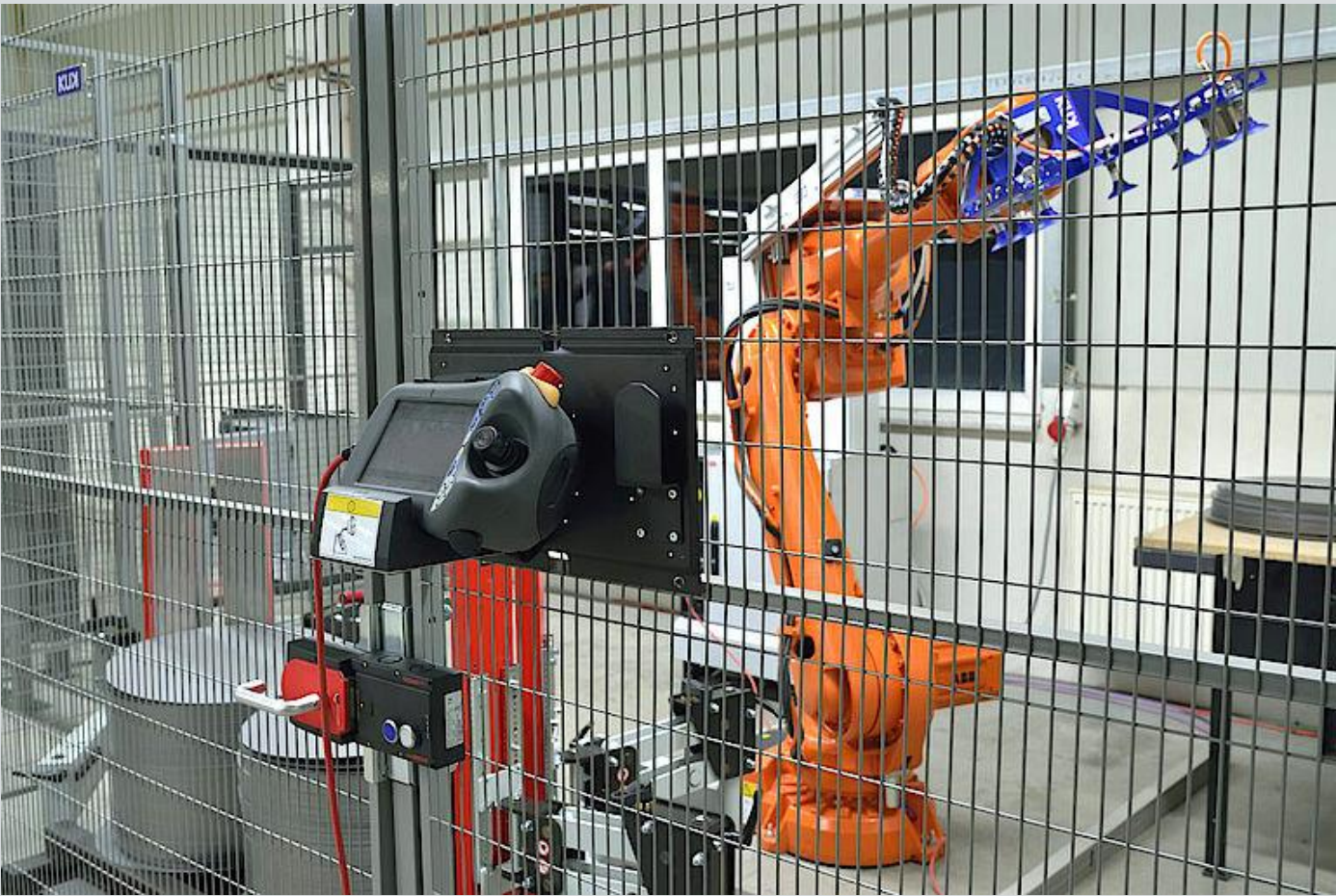
safety cage for an industrial robot
